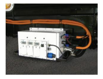
The **Optional 5 KW APG** provides clean sine wave AC power (110V or 208V) for lights, tools, or computers, and has even been integrated with refrigeration systems.
