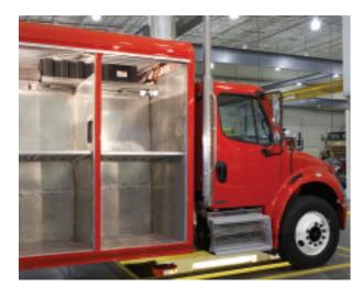
In many applications, **the lithium ion battery** is re-located by the body builder to optimize vehicle capacity.
